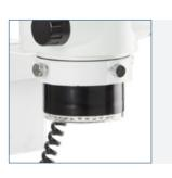
Built-in ring light with 30 intensity adjustable LED's
