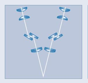
Two optical trains with their optical axes under a small angle generate two images of the object
