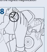
Rotate the diopter adjustment rings of the left and right eyepiece to bring the specimen into focus
