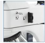
Reflected illumination with rotating color filter disc
