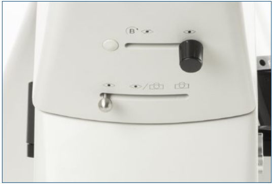
● Bertrand lens and trino/eyepieces selector
